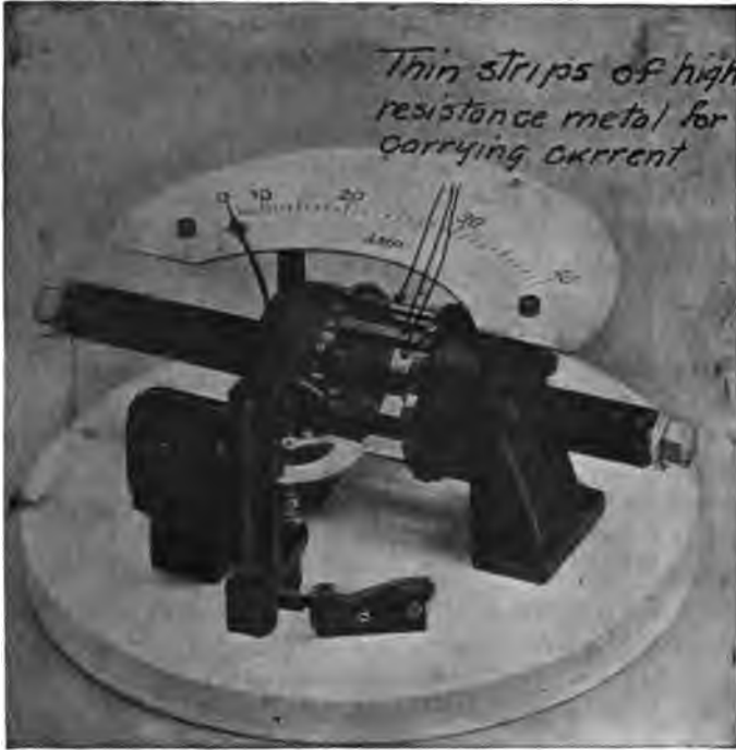
FIG. 12.—A hot wire ammeter showing how the skin effect is minimized by special arrangement of very thin strips of high-resistance metal.
